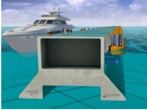
Fig. 3120 Illustration of breakwater structure combining production of energy from attached converters.
