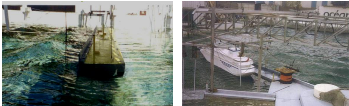
Fig. 21 Testing of floating breakwaters and jetty in laboratory of hydrodynamics. The testing was conducted for Monaco harbour by Dorris Engineering.
